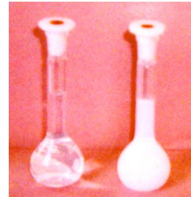
The microemulsion is transparent because the particle size is lower than the light wavelength
